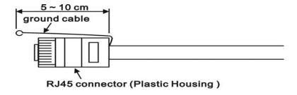
2. Make the ground cable connect to ground screw, then plug RJ45 connector.
