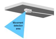
Fix sensor to the surface with screws or Velcro closing, included in the delivery.
