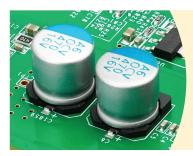
Unlike normal switch hardware design with Electrolytic capacitors (E-cap), the Zyxel Nebula Cloud Managed Switches adopt solid capacitors to get rid of drying out, bursting and leaking problems. Solid capacitors ensure Nebula switches with longer lifetime, high stability and robust operation.
