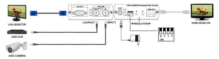
\* 3 outputs: HDMI, VGA, AHD loop output as a distributor.
