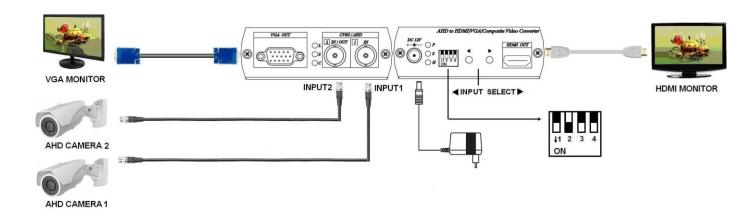
\* Allow AHD camera 2 inputs with 2 outputs: HDMI, VGA as a Switcher.
